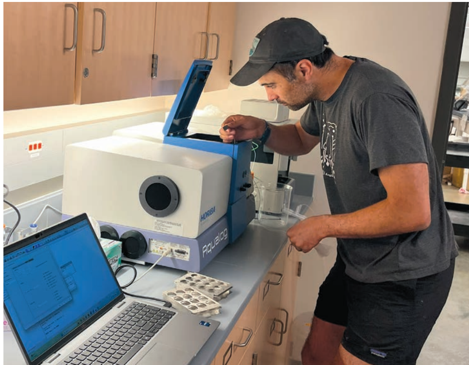
Kyle Shimabuku, Ph.D. uses the Horiba Aqualog to characterize contaminants in wildfire-impacted drinking water sources.
