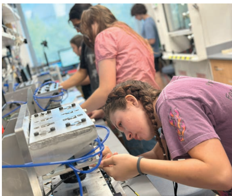
A SSIP student in the Tribology Lab mounting a composite polymer sample for a tribometer wear test.
