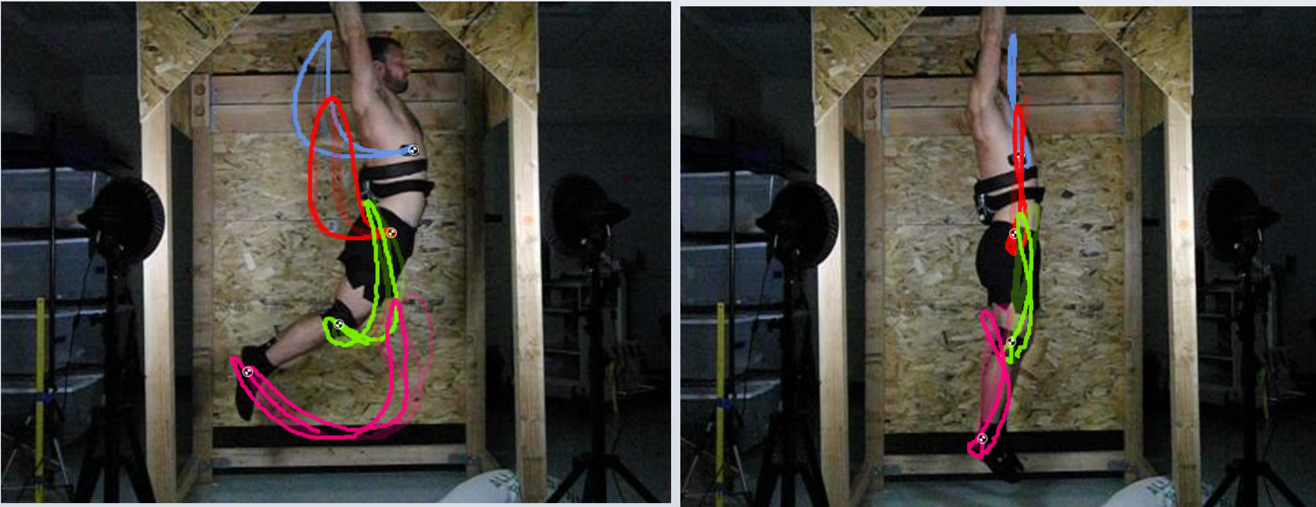
Figures 2 and 3: Motion tracker path of markers for a KPU (left image) and SPU (right image) for Subject 1
