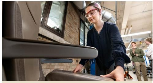
One senior design team redesigned an airplane seat using alternative materials, suppliers, and assembly methods to decrease shipping emissions and in-service fuel consumption while increasing seat durability and use of post-consumer recycled materials.
