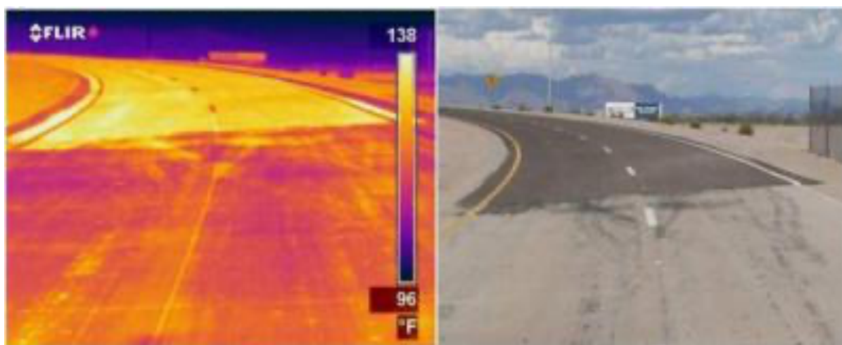
Figure 8 - Thermal infrared (left) and visible (right) images of a road with cool pavements and traditional asphalt. The infrared image shows that the light segment (bottom) is about 30 °F cooler than the dark segment (top).
